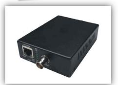
Receiver, without POE function, 1 channel 10/100Mbps IP Ethernet transmission over Coax up to 500m, one coax port to one Ethernet port, input AC110-220V, out DC 5-12V
