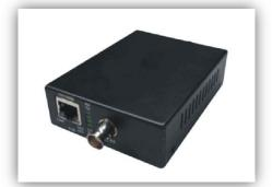
Transmitter, without POE + (30W) to power the IP camera, 1 channel 10/100Mbps IP Ethernet transmission over Coax up to 500m, one coax port to one Ethernet port, input AC110-220V, out DC 48-56V
